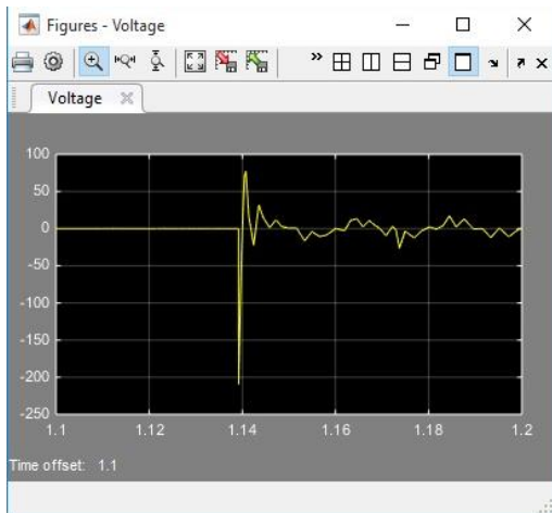
Fig. 6 Voltage variation on coil when connection is initiated
